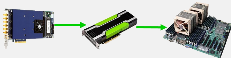
Remote Direct Memory Access (RDMA) transfer digitizer data directly to the GPU for image processing
