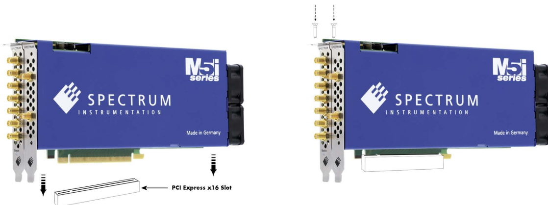
Image 6: Mounting M5i PCIe card into connector
